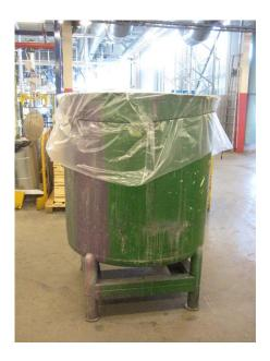
Allied Filter Systems Ltd, in partnership with Buscherhoff Spezialverpacknung GmbH & Co. KG, have developed a range of tank covers manufactured from a new antistatic film designed to virtually eliminate the emission of solvents into the atmosphere.
