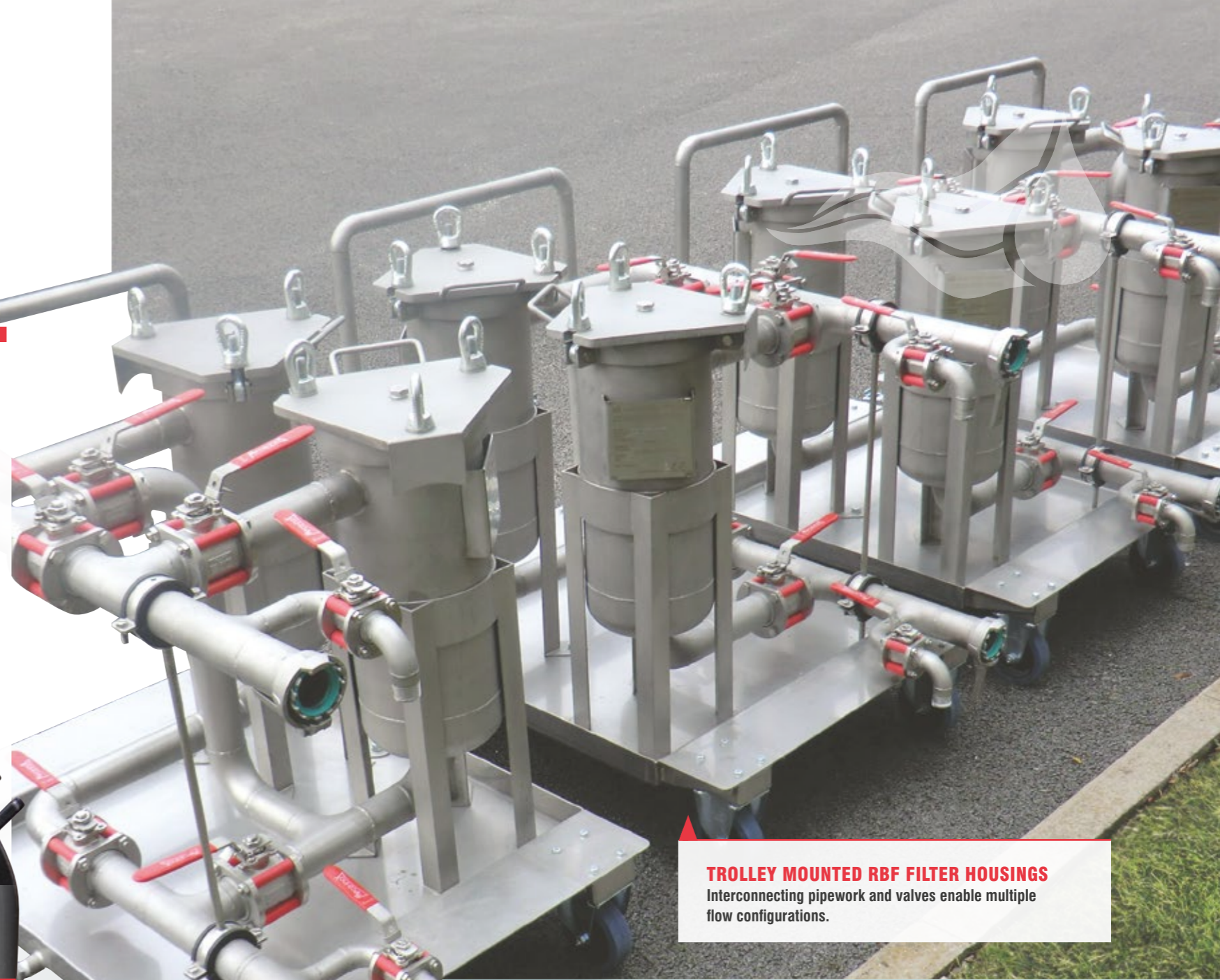
MODULAR SYSTEM with common inlet and outlet pipes. Valves are fitted to enable isolation of individual or multiple housings to enable filter bag change during continuous operation. The number of housings may be increased at any time to expand the system.
