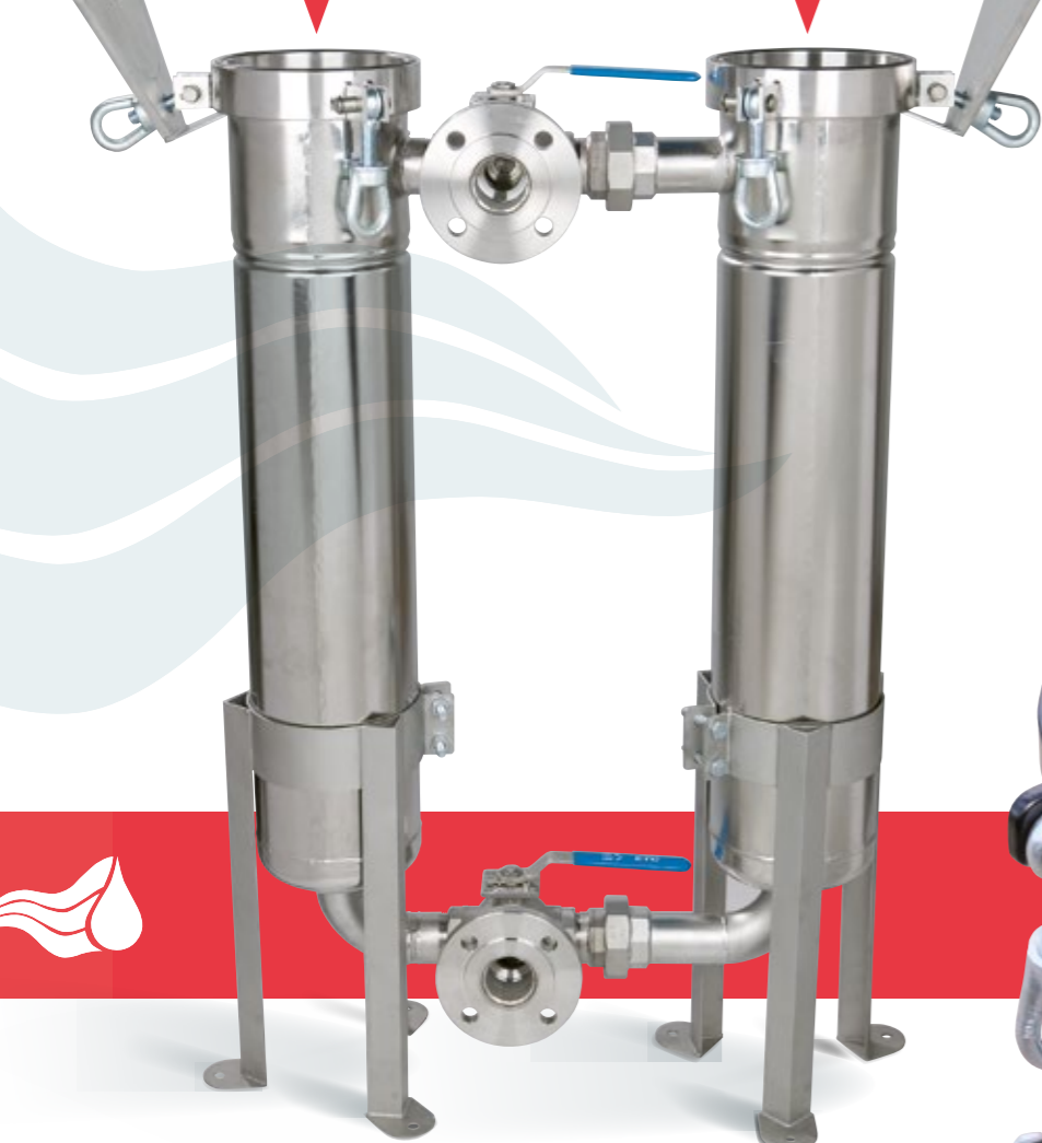
TWO RBFP HOUSINGS manifolded together and fitted with valves to enable use in a continuous process. One filter bag can be changed out whilst the other housing is in use.
