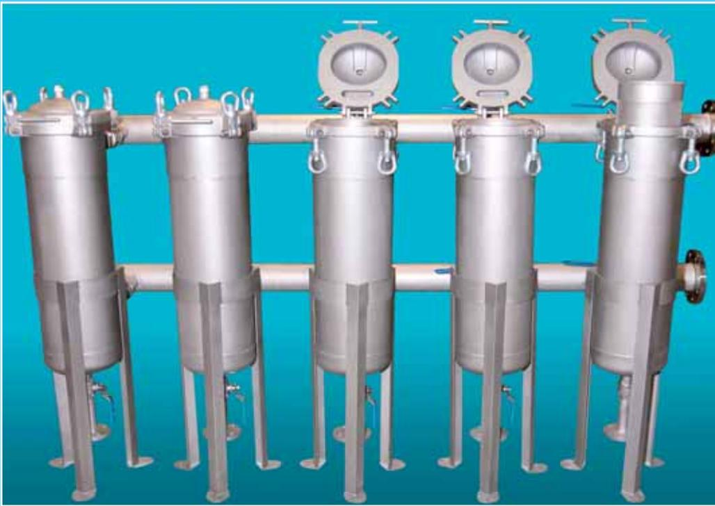
Modular system with common inlet and outlet pipes. Valves are fitted to enable isolation of individual or multiple housings to enable filter bag change during continuous operation. The number of housings may be increased at any time to expand the system
