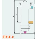
Side inlet - same side outlet - bottom drain. outlet - bottom drain.
