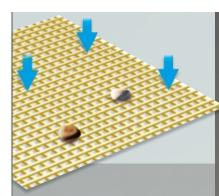
Mesh filter bags provide surface filtration - a 'sieving' mechanism, causing particles larger than the pore size of the media to be captured on the surface of the media.
